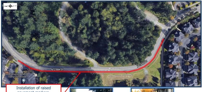
pavement markers, additional signage, and enhanced pavement lane striping
